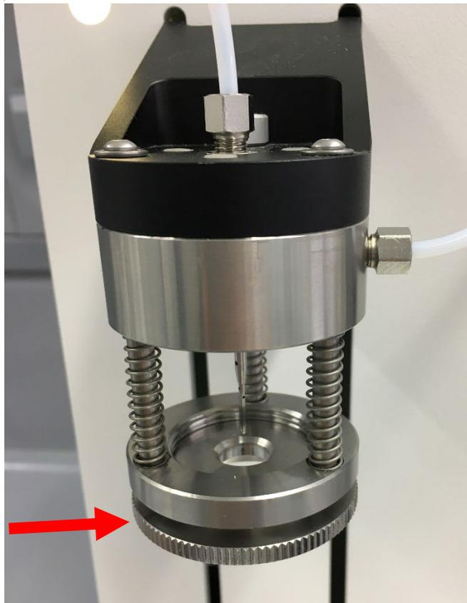
The needle can then be unscrewed with the needle wrench (special tool, included with the TO 7280):
